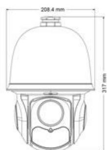
**2 Megapixel Starlight HD Analog IR PTZ Speed Dome Kamera**
